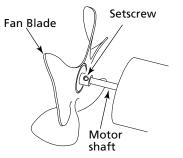
Figure 6 - Fan, Motor Shaft, and Setscrew Location
